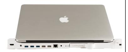
This is looking from the rear of the laptop. You gain some extra ports and it needs a power supply for the USB 3.0 ports, if you tend to charge your iPhone. Please note that the max amp is 0.9 mA, so it's not a fast charger! It has an ether port but it did not work. So I had to do a little homework on WHY?
